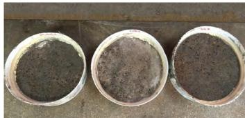
(top to bottom) Of 100 ml of oil poured onto cement, EnBio absorbed the least, 21 ml, after 24 hr. From left to right are mineral oil, EnBio and a vegetable oil blend.
